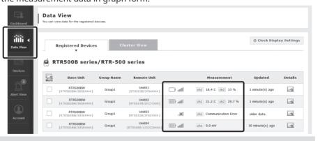
The signal strength between Base Unit and Remote Unit can be checked by color and number of antennas. When using Repeaters, the signal strength displayed here is only that for between the Remote Unit and the nearest Repeater. To check the signal strength between the Base Unit and Repeater or between Repeaters, please use the
